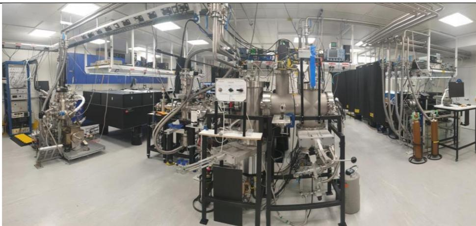
Photoelectron spectroscopy end-stations in the new Ultrafast Laser Facility. Left to right: UHV hemispherical analyser photoelectron spectrometer for surface science studies, liquid-microjet magnetic bottle photoelectron spectrometer, molecular-beam photoelectron velocity-map imaging (VMI) spectrometer, electrospray ionisation VMI spectrometer).
