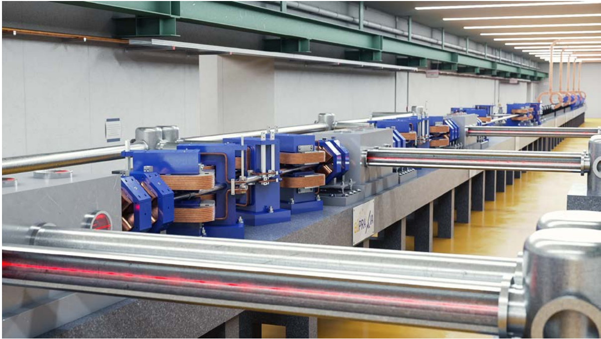
Rendering of the two-stage, very low energy spread plasma accelerator developed for the EuPRAXIA facility. The open tubes show the paths of the laser pulses (red lines) that drive the plasma wakefields in the vacuum chambers.
