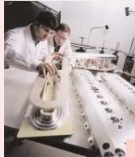
Engineers examining the high-temperature superconducting coil for a 1000-hp motor
