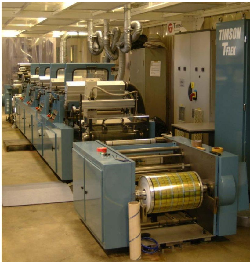
Timsons T-flex 508 flexographic press for functional printing at the Welsh Centre of Printing and Coating, Swansea University. Image credit: Alan Hodgson
