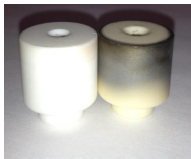
Figure 2 New versus after-life insulators
