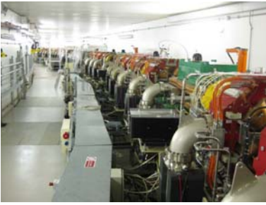
Fig 1: View in the Diamond storage ring tunnel . The electromagnets focus and deflect the stored electron beam (green, red and yellow in coloured version). The large elbows which connect the vacuum vessels to the ion pumps are clearly visible.
