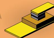
*The single cell of an MRAM using a magnetic tunnel junction*
