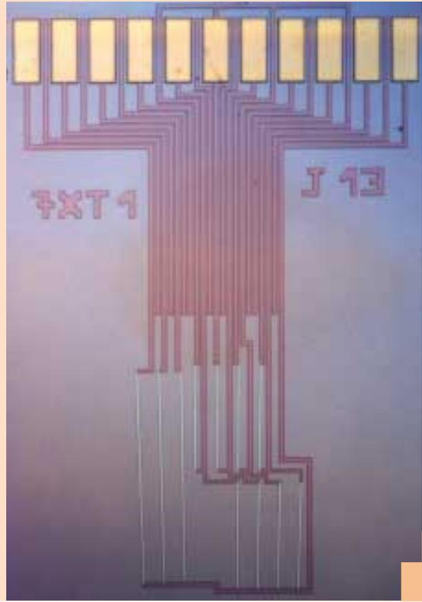
A magnetic field sensor made of GMR multilayers (iron-nickel with silver) for an angular encoder
