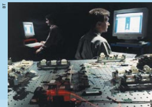
BT's quantum cryptography system. The two computers are connected by 28 kilometres of optical fibre in the Ipswich area of BT's public network
