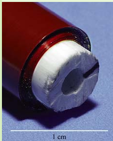
A single element showing the Swiss roll structure that gives rise to a negative magnetic response
