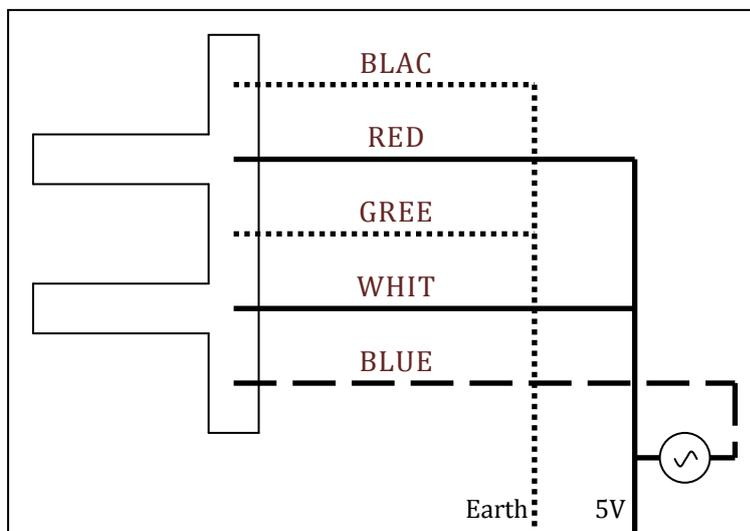
Figure 4.1: Diagram depicting the correct set-up for the Light Gates including the attachment to the Oscilloscope
