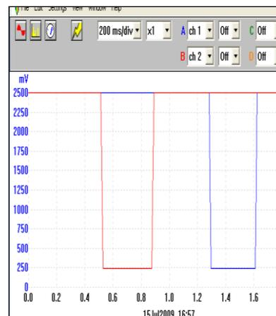
Figure 4.2: Oscilloscope readings as the train passes through both gates
