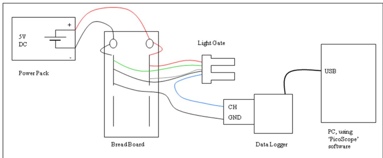
Figure 4.3: Light gate wiring.
