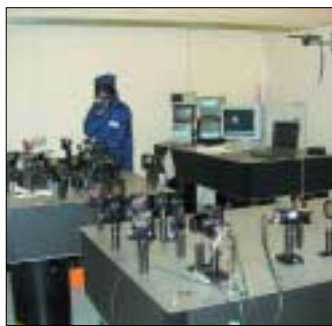
Jodie Smith uses an infrared viewer to examine a sample of the Vulcan petawatt laser beam as it travels through a custom diagnostic system.
