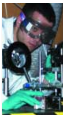
Andy Bodey makes adjustments to a spatial filter that is used to improve the beam quality of the laser-plasma X-ray laboratory's high-power, ultraviolet excimer laser.
