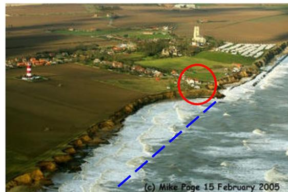
Figure 3 – Coastal erosion forming a bay at Happisburgh, Norfolk. The blue line indicates the position of the cliff before the defences started to fail in 1996. Miss Wrightson's tea shop (circled in red) is dangerously near the cliff edge. Photograph taken by Mike Page, 15<sup>th</sup> February 2005.
