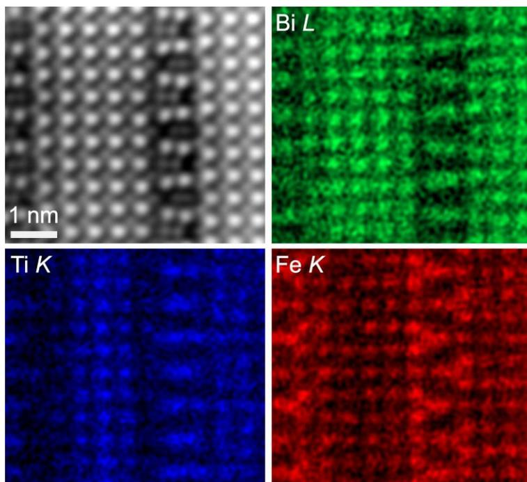
HAADF-STEM image (top left) and STEM-EDX maps of a bismuth ferrite-lead titanate thin film analysed by a non-aberration corrected, FEI Titan Themis G2 300 (sample prepared by Dr Faye Esat, images courtesy of Dr Andy Brown, University of Leeds).
