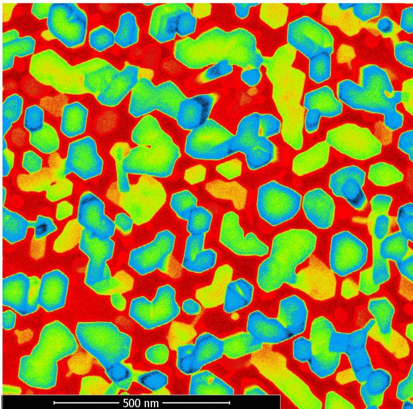
*False colour secondary electron SEM image of GaN nanowires
