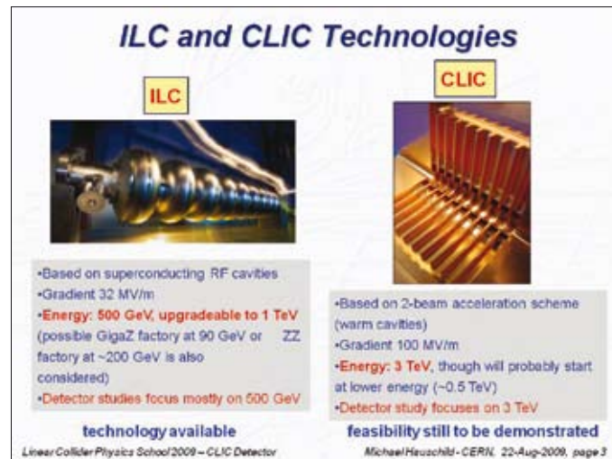
A comparison of the technologies of the proposed superconducting International Linear Collider and CERN's Compact Linear Collider.
