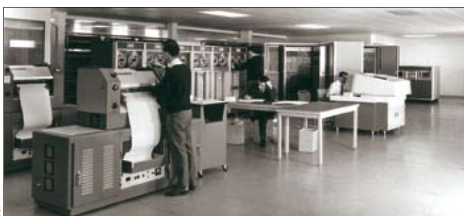
General view of the original 6600 computer room at CERN. The computer is in the background and the tape units can also be seen.
