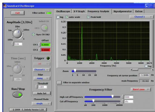
Figure 2. ‘Overblowing’ eliminates the fundamental (~600 Hz) so the main frequency heard is then around 1200 Hz (one octave higher).
