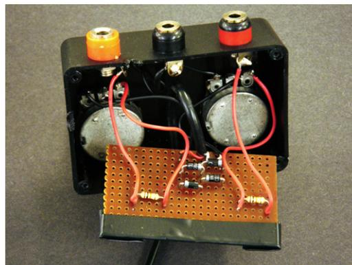
**Figure 4.** Soundcard input device, showing back-to-back diodes.
