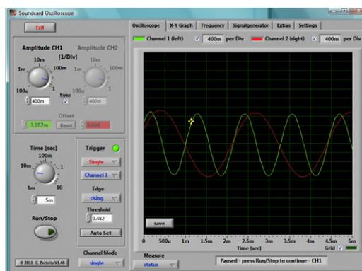
**Figure 5.** ‘Scope’ software in use as a dual-beam oscilloscope.
