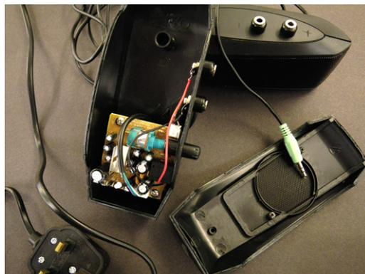
Figure 6. Loudspeaker-turned-signal-generator.
