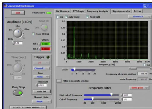
Figure 1. Zeitnitz’s ‘Scope’ software being used for frequency analysis.
